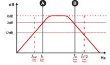
To set the "HIGH" variable control between 5Hz and 80Hz ("A") where you want to perform the subsonic cut filter;
