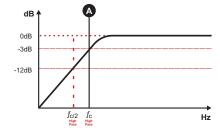
Set in the "LOW PASS" variable control between 80Hz and 20kHz ("B") where you want to perform the low pass cut filter;
