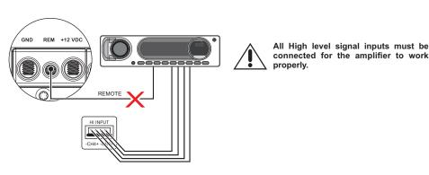
High level input must be used when the main unit does not have RCA outputs.
