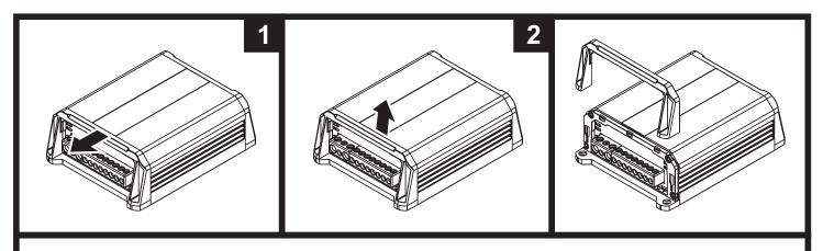
1. Carefully pull out the top of the plastic cover to release the upside latches, as shown in picture 1.2. Slide up the plastic cover in a continuous movement to remove it.
