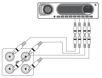
All RCA inputs must be connected for all 4 channels to work.
