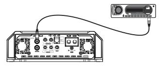
Example of two RCA cables connection (mono input).
