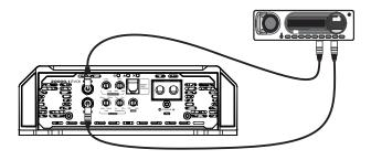
Example of one RCA cable connection only and using the RCA output to connect another amplifier.
