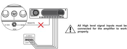
High level input must be used when the main unit does not have RCA outputs.
